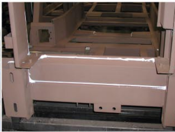
LoVOC Seal used for weldline and crevice sealing bus frame
